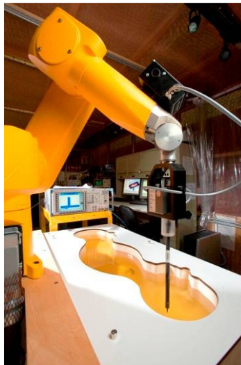
Figure 3-2 DASY4 SAR Measurement System
