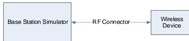
Figure 14-1 Power Measurement Setup
