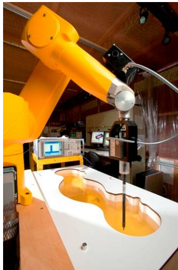
Figure 3-2 DASY4 SAR Measurement System
