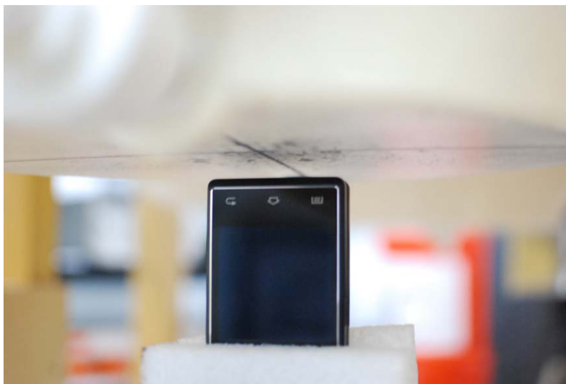
SAR Test Setup Photo 8: Bottom at 1.0 cm
