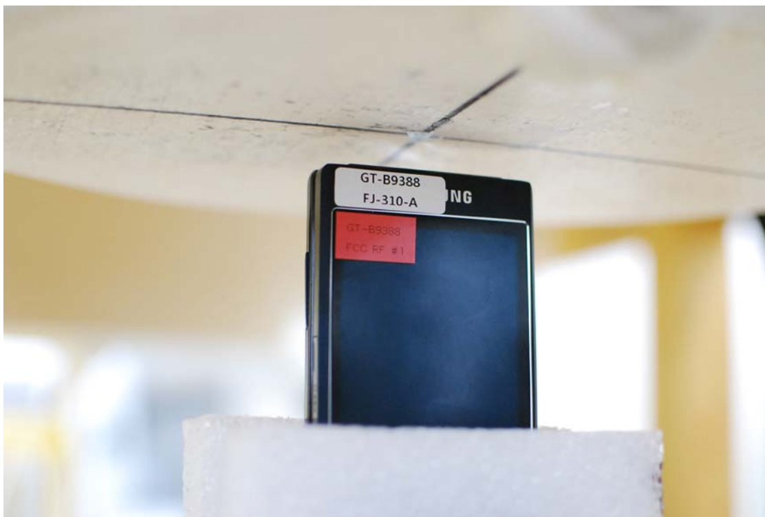
SAR Test Setup Photo 7: Top at 1.0 cm
