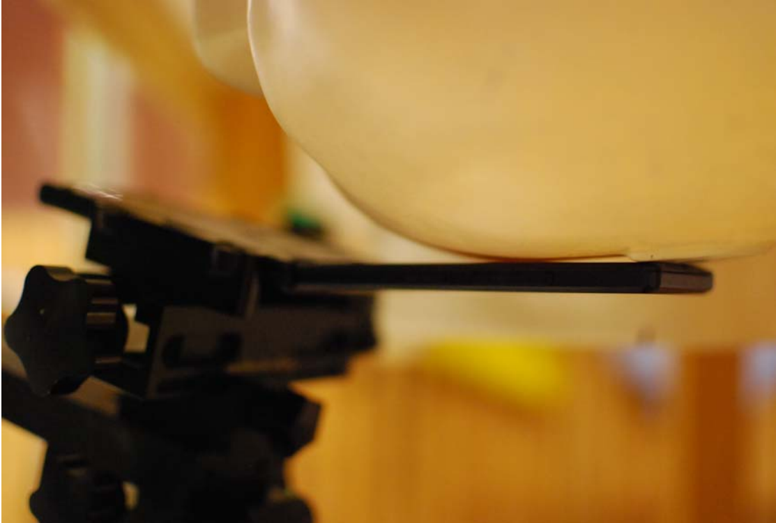
SAR Test Setup Photo 3: Left Cheek
