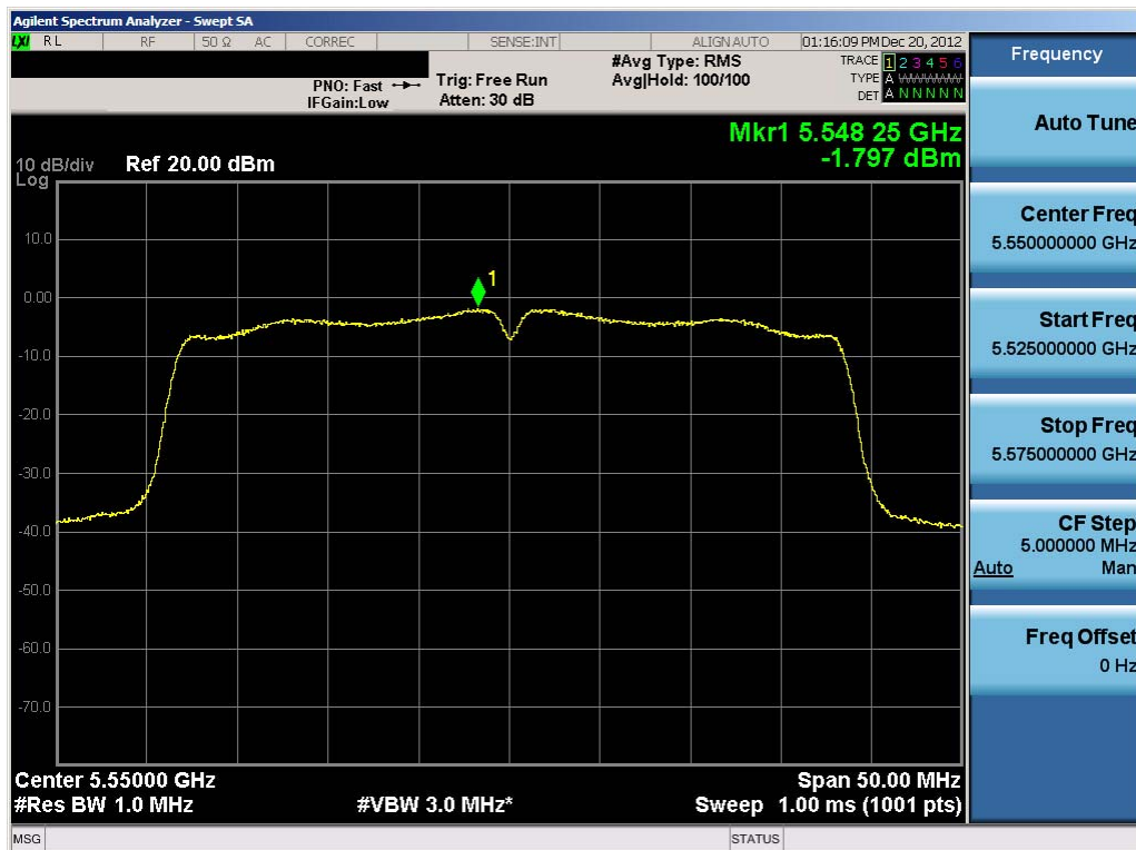
Plot 6-49. Peak Power Spectral Density Plot (40MHz BW 802.11n (UNII Band 3) – Ch. 110)
