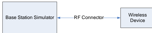
Figure 14-1 Power Measurement Setup
