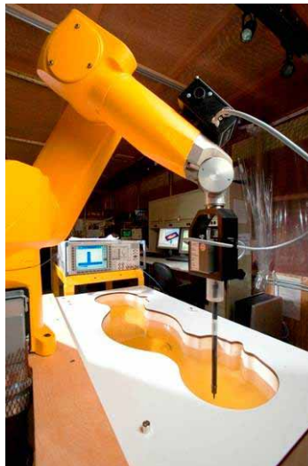
Figure 3-2 DASY4 SAR Measurement System
