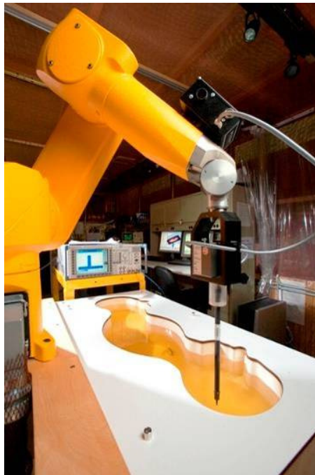
Figure 3-2 SAR Measurement System
