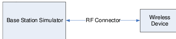
Figure 11-1 Power Measurement Setup
