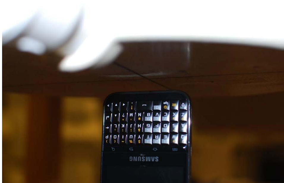
Figure 21-8 SAR Test Setup Photo 8 – Bottom at 1.0 cm
