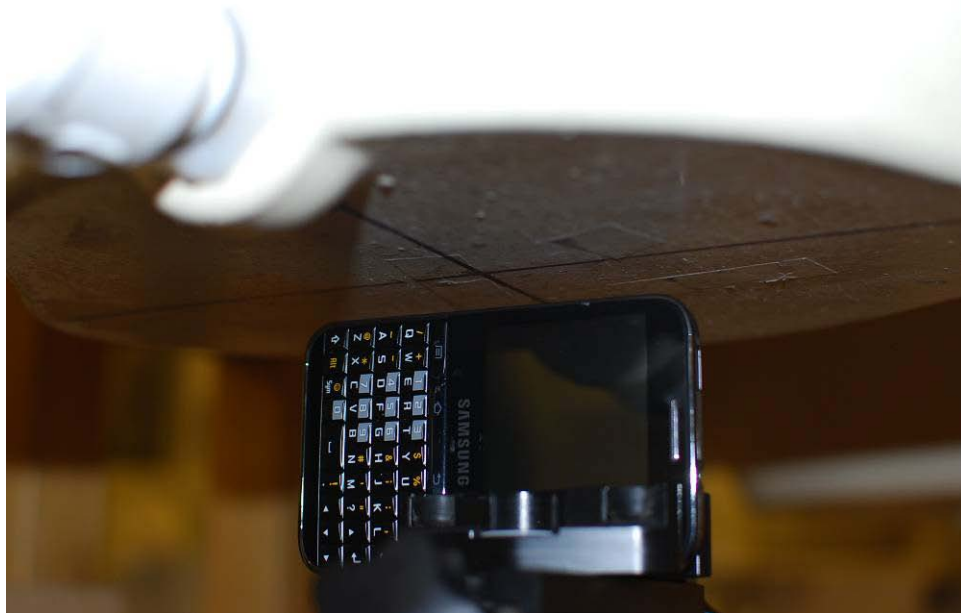
Figure 21-10 SAR Test Setup Photo 10 – Left at 1.0 cm
