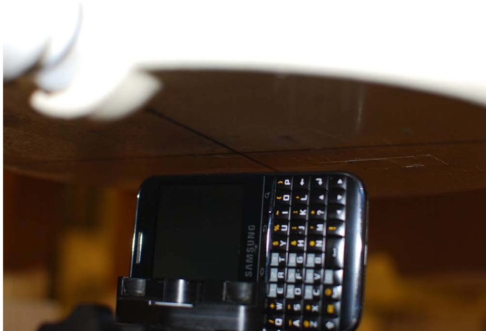
Figure 21-9 SAR Test Setup Photo 9 – Right at 1.0 cm
