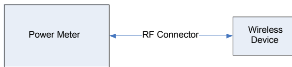
Figure 12-1 Power Measurement Setup
