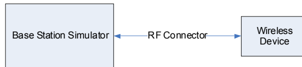
Figure 11-1 Power Measurement Setup
