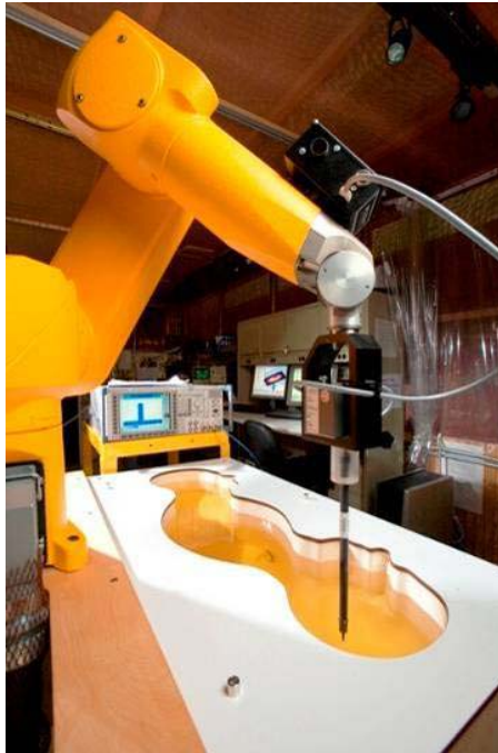
Figure 3-2 SAR Measurement System
