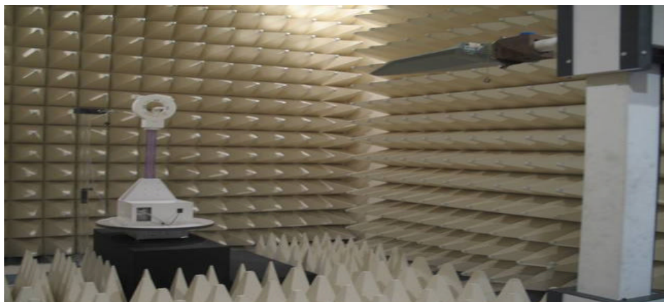
Figure2. Photograph of 3m Fully-Anechoic Chamber
