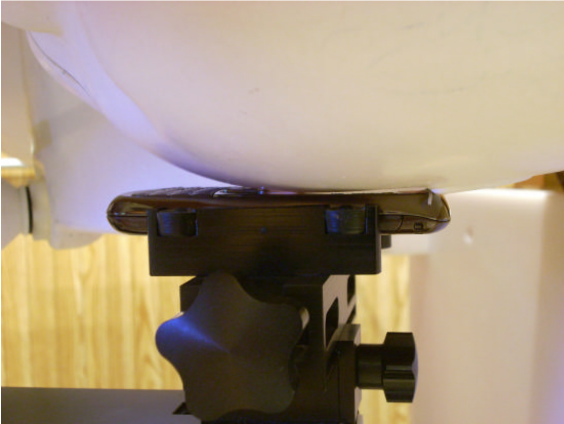
Figure 5: Left Head SAR, Cheek Touch
