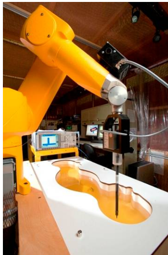
Figure 3-2 DASY4 SAR Measurement System
