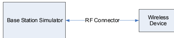
Figure 14-1 Power Measurement Setup
