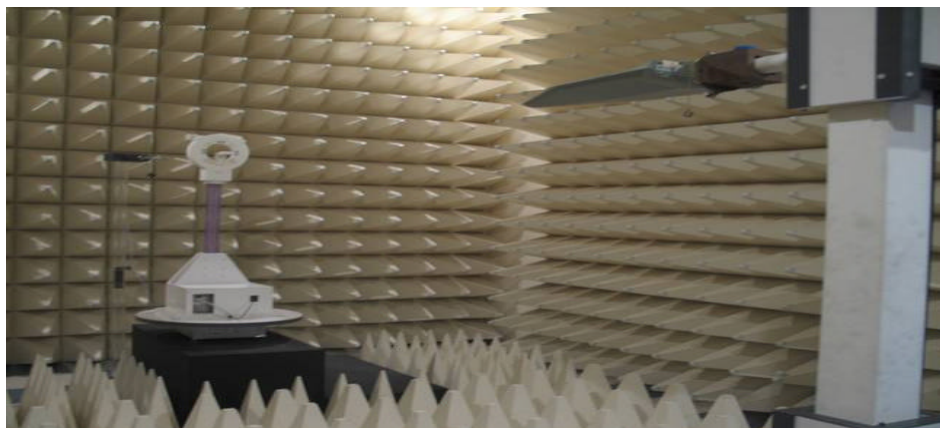
Figure2. Photograph of 3m Fully-Anechoic Chamber
