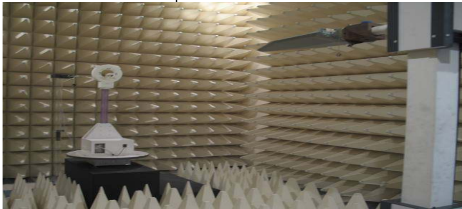
Figure2. Photograph of 3m Fully-Anechoic Chamber
