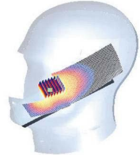
Figure 7-1 Sample SAR Area Scan
