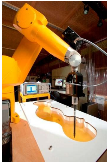
Figure 3-2 DASY4 SAR Measurement System
