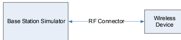
Figure 14-1 Power Measurement Setup
