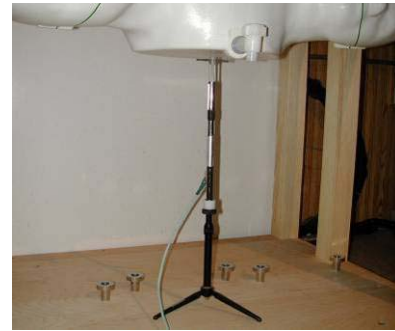
Figure 12-2 System Verification Setup Photo
