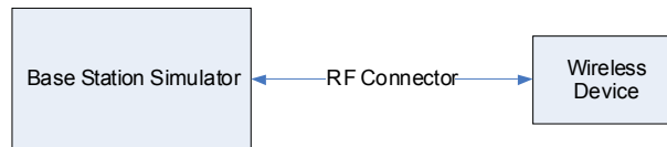
Figure 15-1 Power Measurement Setup
