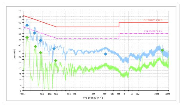
Note 1) Two graphs measured for both Live(L1) and Neutral(N) of the LISN are combined into one graph.
