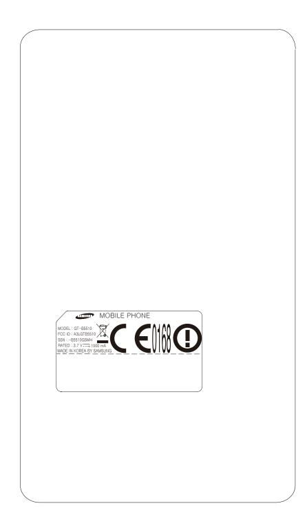
The label is placed inside battery compartment
