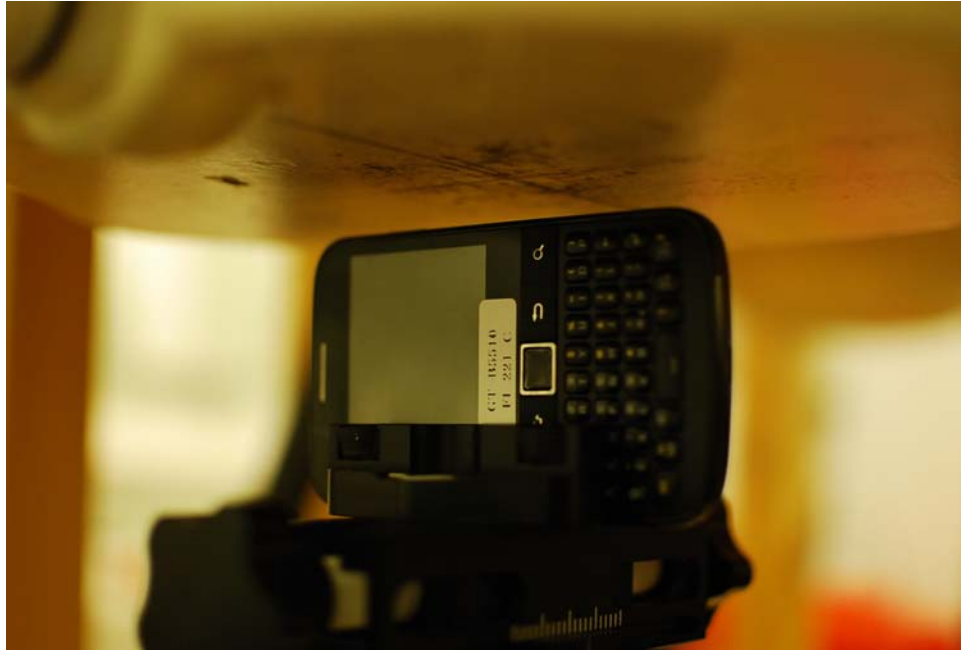
SAR Test Setup Photo 9: Right at 1.0 cm
