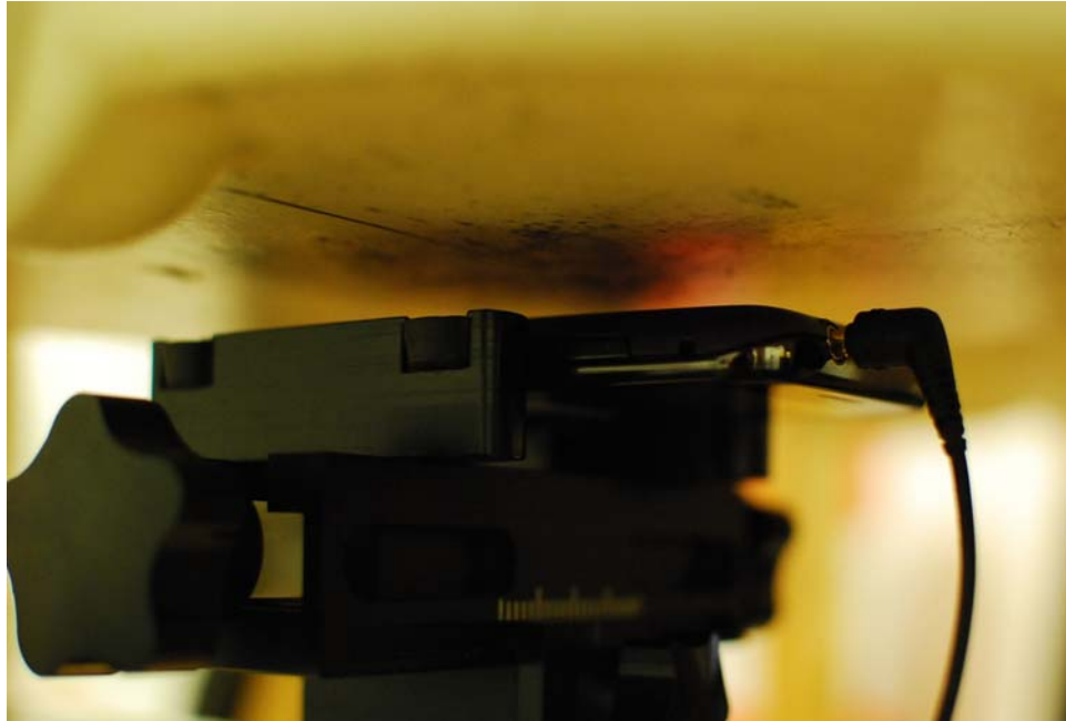
SAR Test Setup Photo 11: Body-Worn at 1.0 cm
