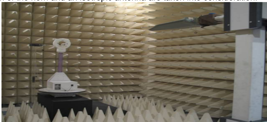
Figure2. Photograph of 3m Fully-Anechoic Chamber
