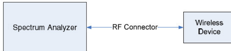
Figure 7-1. Test Instrument & Measurement Setup
