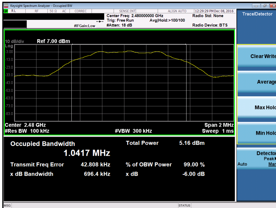
Plot 7-3. 6dB Bandwidth Plot (Bluetooth (LE) – Ch. 39)
