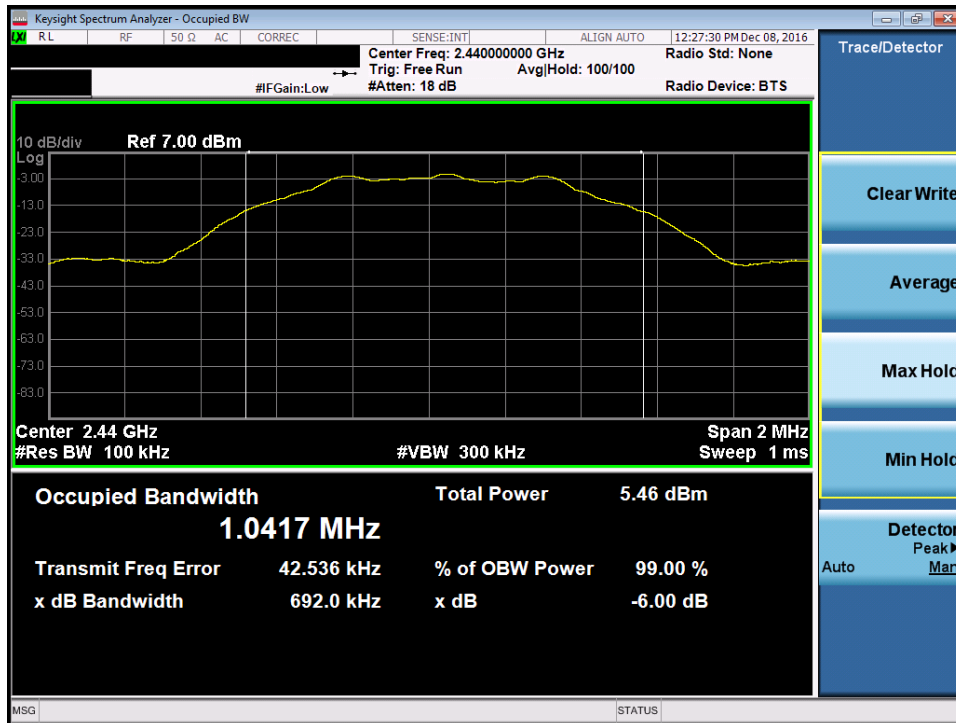
Plot 7-2. 6dB Bandwidth Plot (Bluetooth (LE) – Ch. 19)
