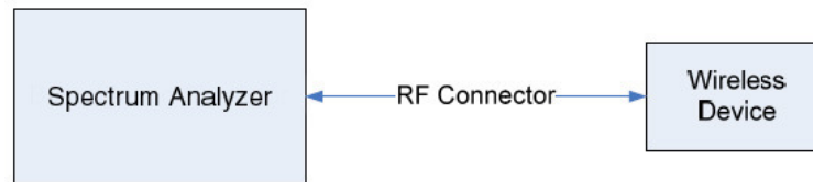
Figure 7-1. Test Instrument & Measurement Setup
