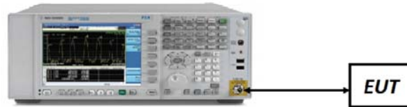
Figure 7-1. Test Instrument & Measurement Setup
