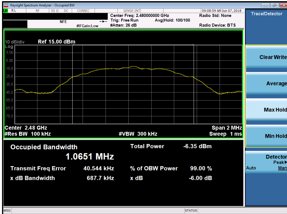
Plot 7-3. Occupied Bandwidth Plot (Bluetooth (LE) – Ch. 39)
