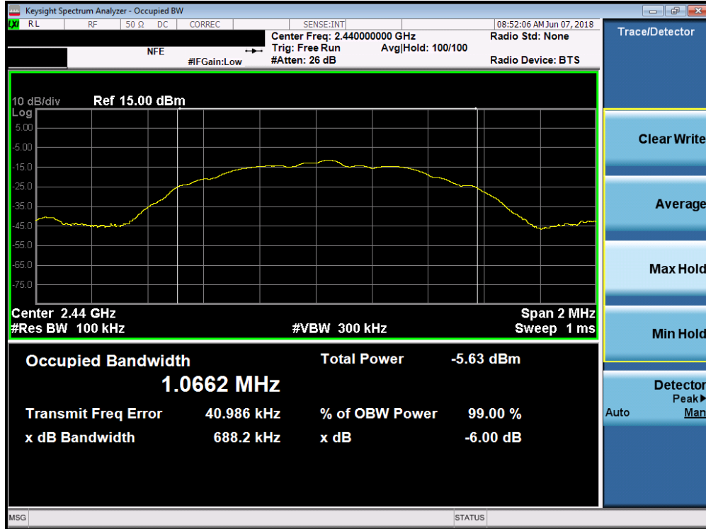
Plot 7-2. Occupied Bandwidth Plot (Bluetooth (LE) – Ch. 19)
