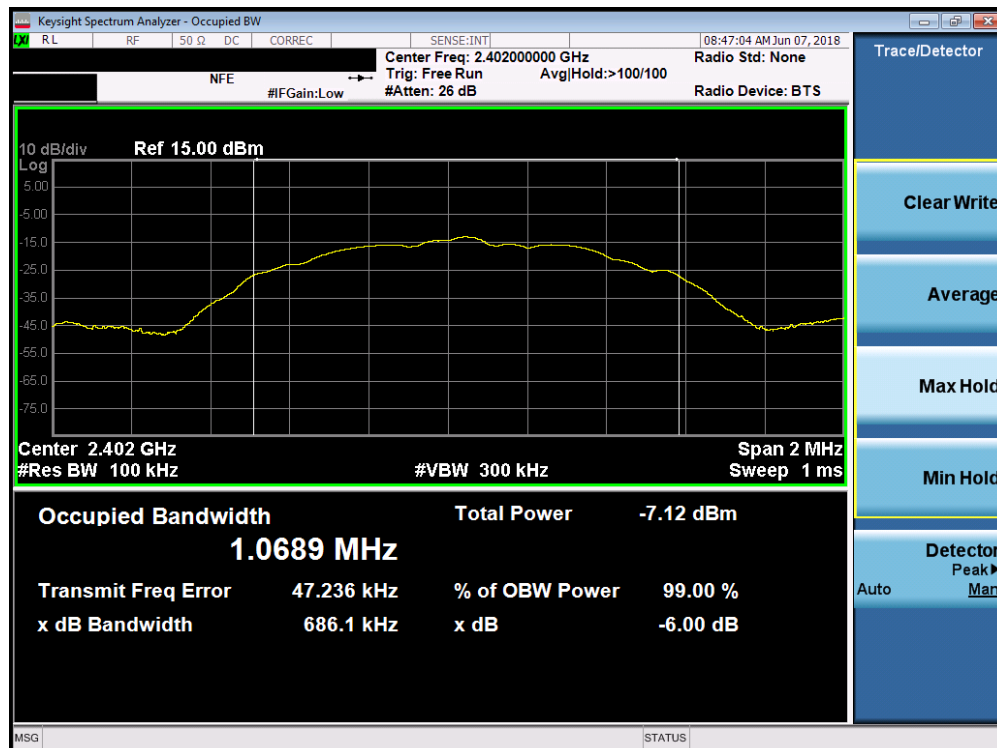
Plot 7-1. Occupied Bandwidth Plot (Bluetooth (LE) – Ch. 0)
