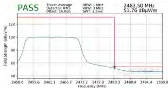
Plot 7-103. Radiated Restricted Upper Band Edge Measurement SISO ANT1 (Average)
