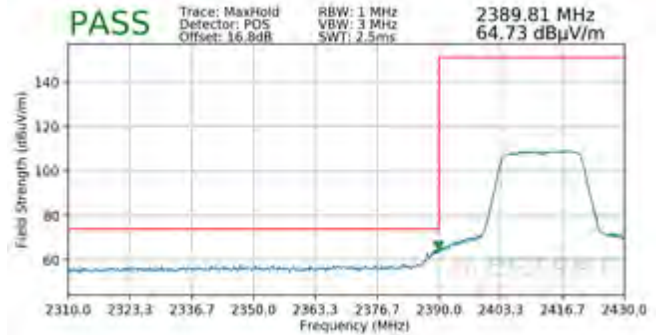
Plot 7-110. Radiated Restricted Lower Band Edge Measurement SISO ANT2 (Peak)
