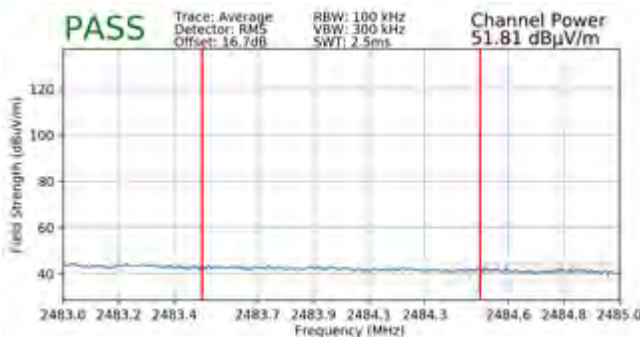
Plot 7-123. Radiated Restricted Upper Band Edge Measurement MIMO (Average)
