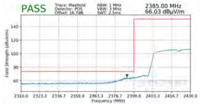
Plot 7-114. Radiated Restricted Lower Band Edge Measurement SISO ANT2 (Peak)
