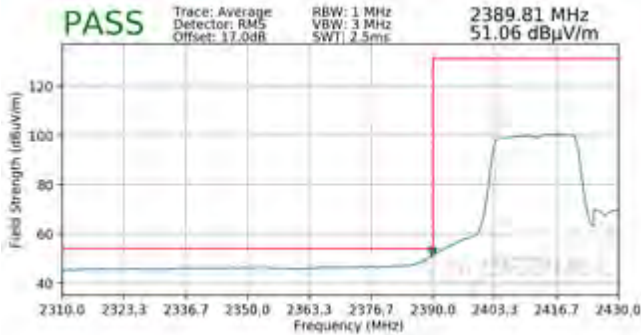
Plot 7-109. Radiated Restricted Lower Band Edge Measurement SISO ANT2 (Average)
