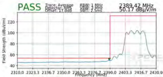
Plot 7-125. Radiated Restricted Lower Band Edge Measurement CDD (Average)
