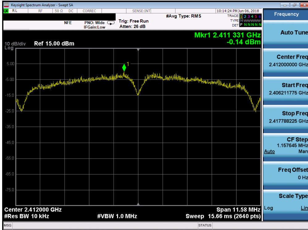
Plot 7-46. Power Spectral Density Plot SISO ANT2 (802.11b – Ch. 1)
