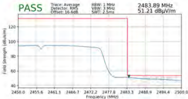
Plot 7-107. Radiated Restricted Upper Band Edge Measurement SISO ANT1 (Average)
