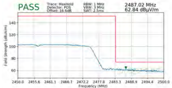
Plot 7-108. Radiated Restricted Upper Band Edge Measurement SISO ANT1 (Peak)
