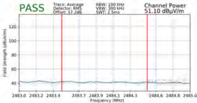
Plot 7-111. Radiated Restricted Upper Band Edge Measurement SISO ANT2 (Average)
