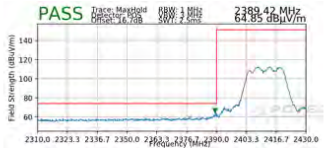
Plot 7-126. Radiated Restricted Lower Band Edge Measurement CDD (Peak)
