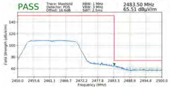
Plot 7-112. Radiated Restricted Upper Band Edge Measurement SISO ANT2 (Peak)
