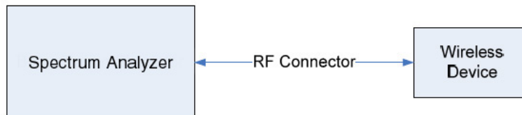
Figure 7-2. Test Instrument & Measurement Setup
