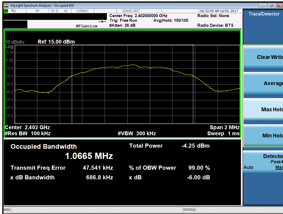
Plot 7-1. 6dB Bandwidth Plot (Bluetooth (LE) – Ch. 0)
