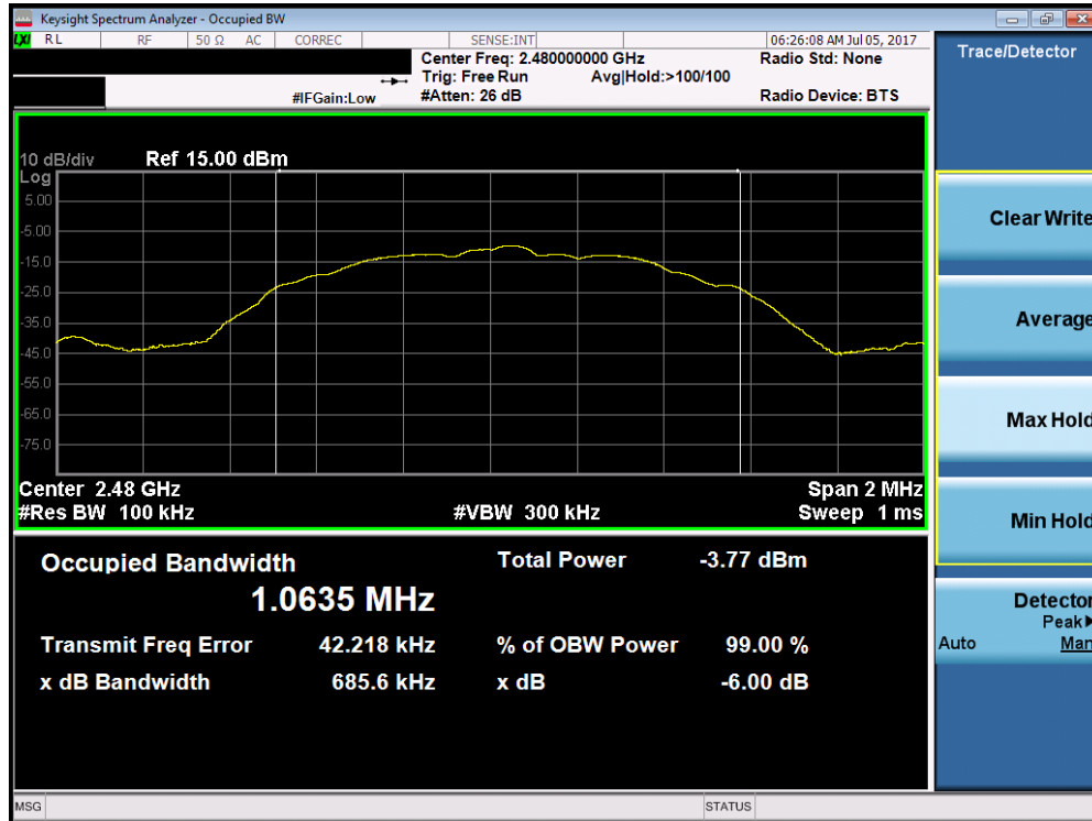
Plot 7-3. 6dB Bandwidth Plot (Bluetooth (LE) – Ch. 39)
