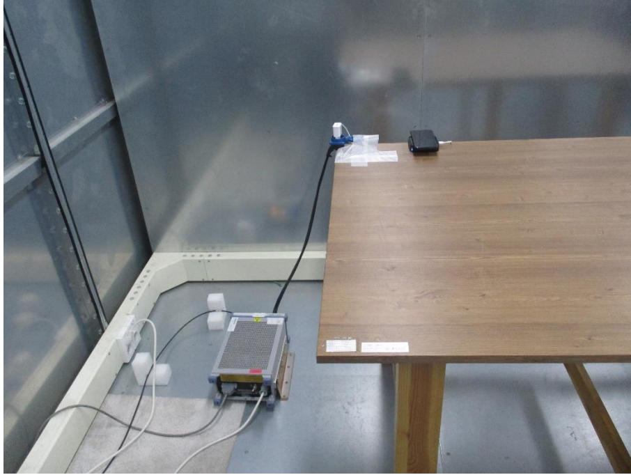
AC LINE CONDUCTED FRONT TEST PHOTO (WPT – worst case 15 Watt)
