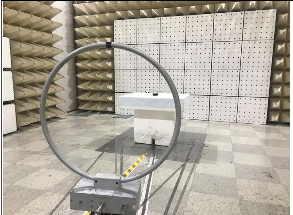
Photo of Test Set up (9 kHz ~ 30 MHz)
