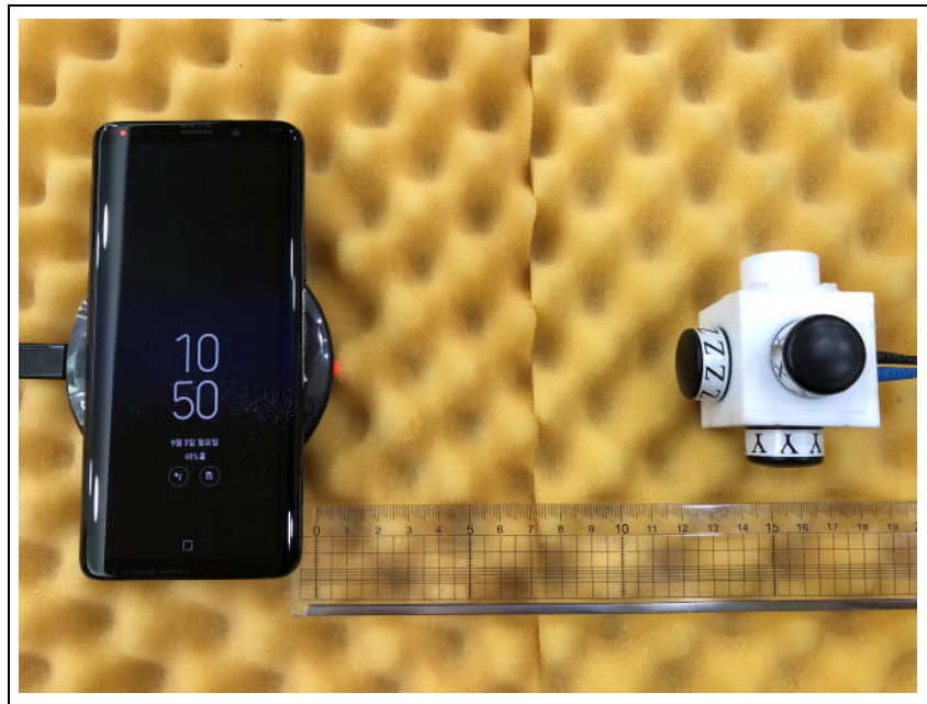
Photo of MPE Test Set up (E-field)
