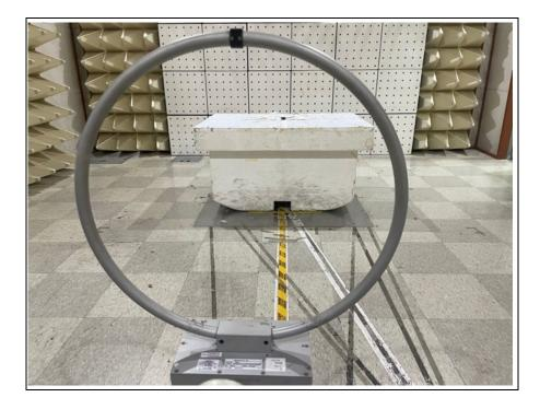
3. Photo of Radiated Spurious Emission Test (30 Mz ~ 1 000 Mz)
