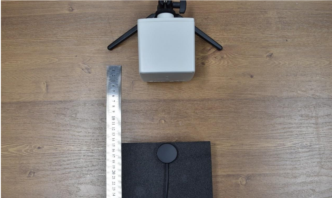
S1, RF EXPOSURE SETUP PHOTO @15cm
