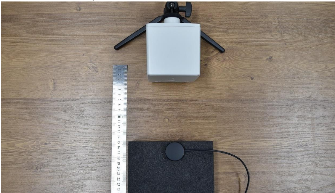
S2, RF EXPOSURE SETUP PHOTO @15cm
