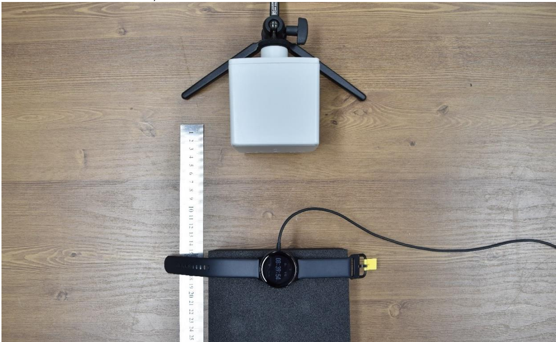
S3, RF EXPOSURE SETUP PHOTO @15cm
