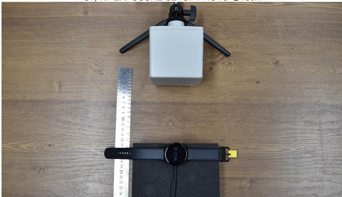
S1, RF EXPOSURE SETUP PHOTO @15cm
