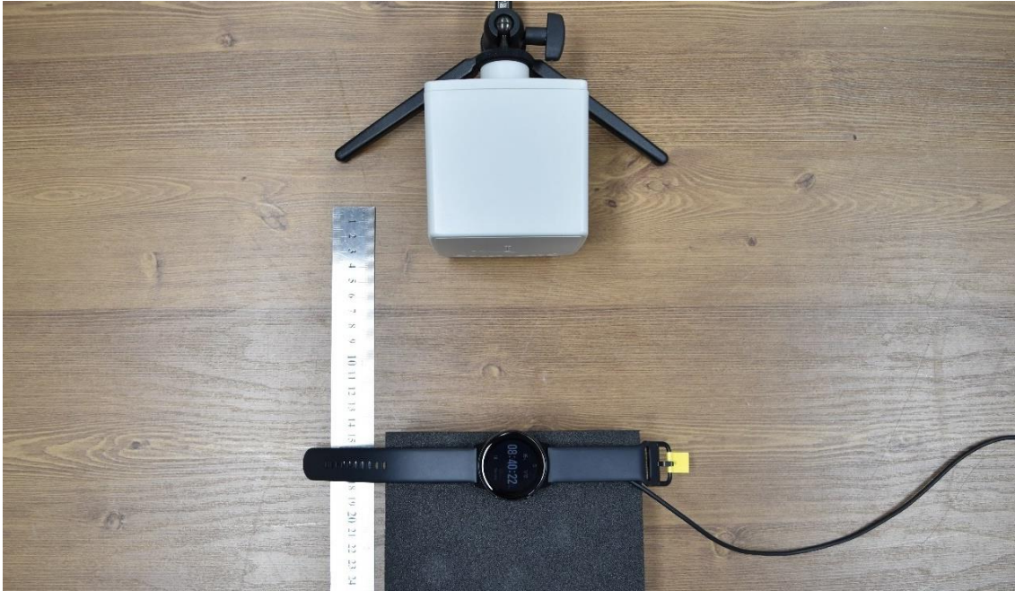
S3, RF EXPOSURE SETUP PHOTO @15cm
