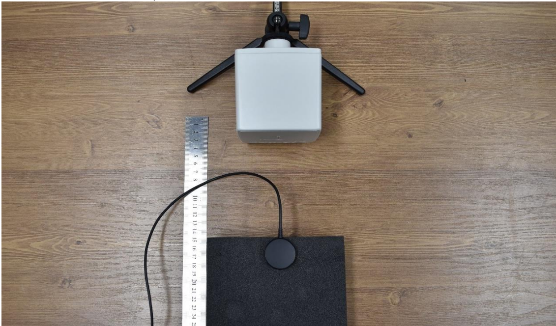
S4, RF EXPOSURE SETUP PHOTO @15cm
