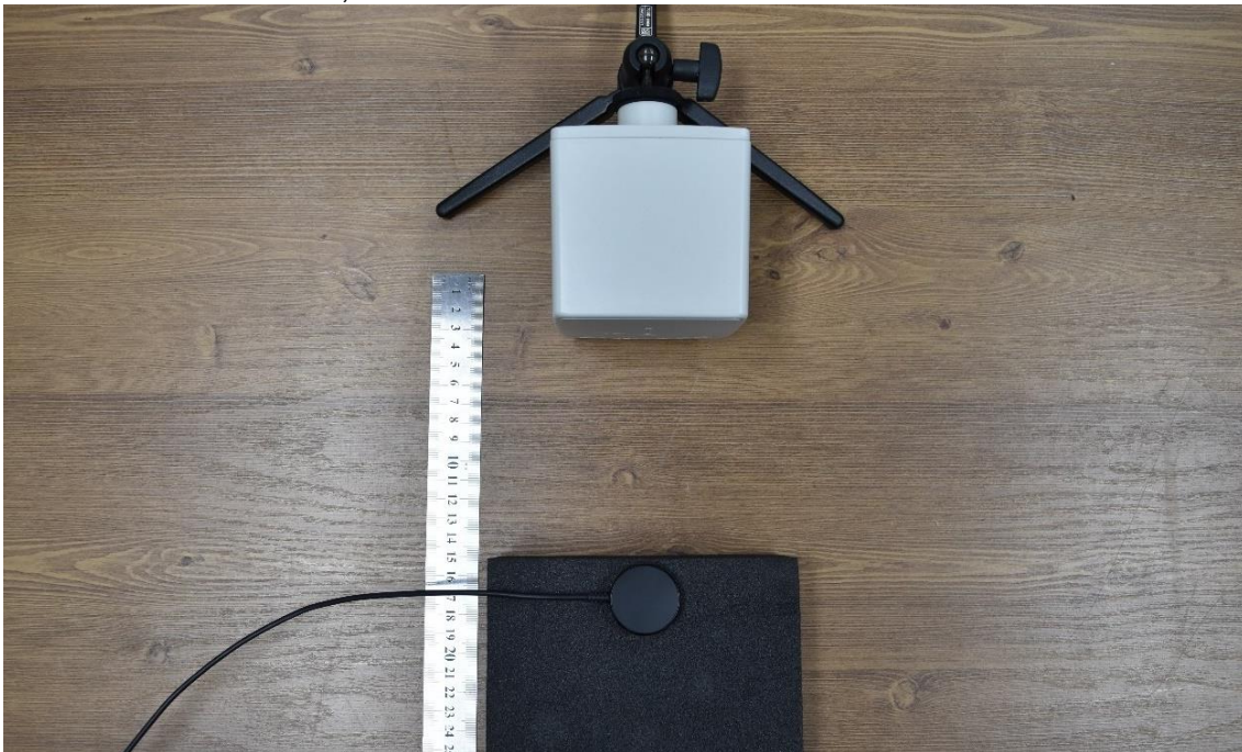
S4, RF EXPOSURE SETUP PHOTO @15cm
