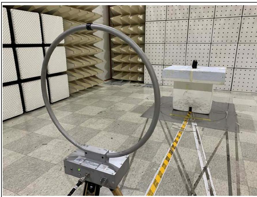
**3. Photo of Radiated Spurious Emission Test (30 MHz ~ 1 000 MHz)**
