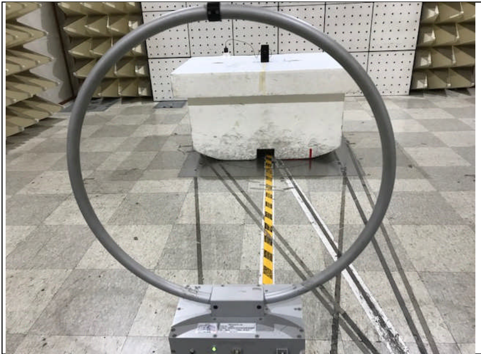
Photo of Test Set up (9 kHz ~ 30 MHz)
