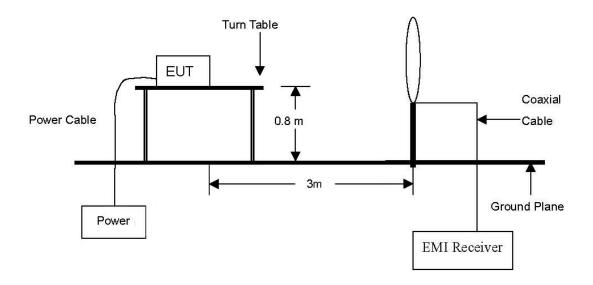
The diagram below shows the test setup that is utilized to make the measurements for emission from 30  $\,\mathrm{Mb}$  to 1  $\,\mathrm{Ghz}$ .
