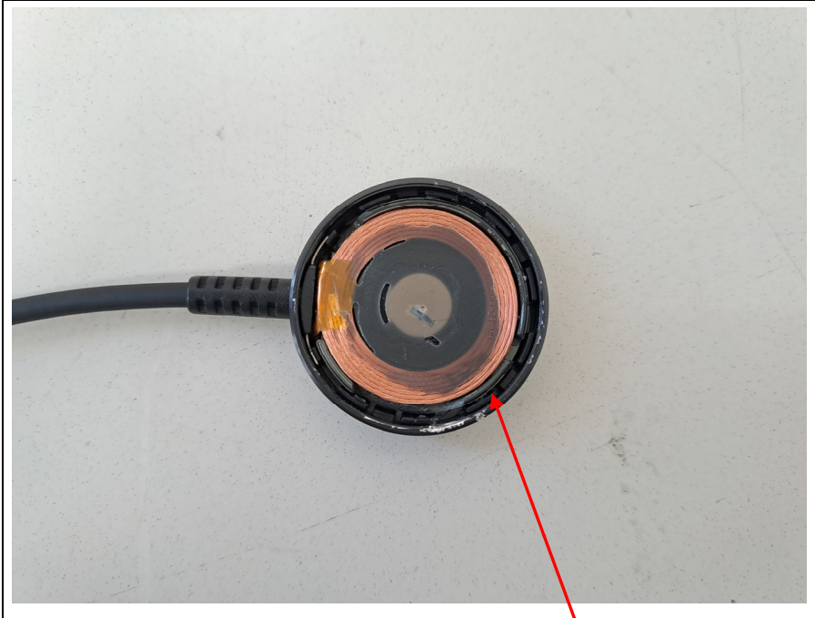
Loop coil antenna
