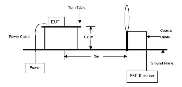
The diagram below shows the test setup that is utilized to make the measurements for emission from 30  $\,\mathrm{Mz}$  to 1  $\,\mathrm{Gz}$ .
