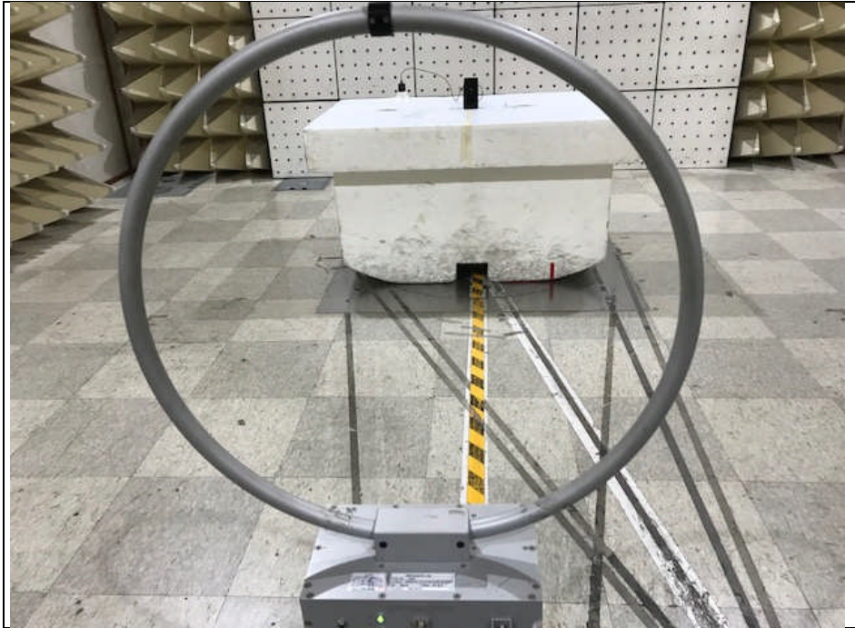
Photo of Test Set up (9 kHz ~ 30 MHz)
