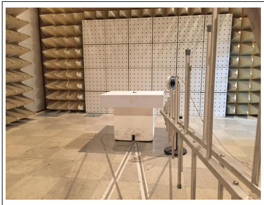
**B. Photo of Radiated Spurious Emission Test (Above 1 GHz)**
