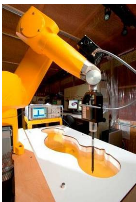
Figure 3-1 SAR Measurement System
