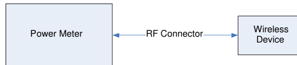
Figure 8-2 Power Measurement Setup
