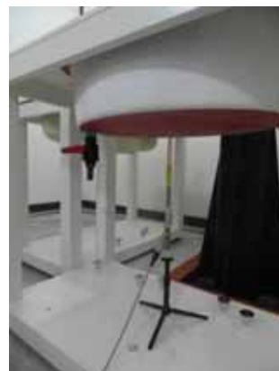
Photo of the dipole Antenna
