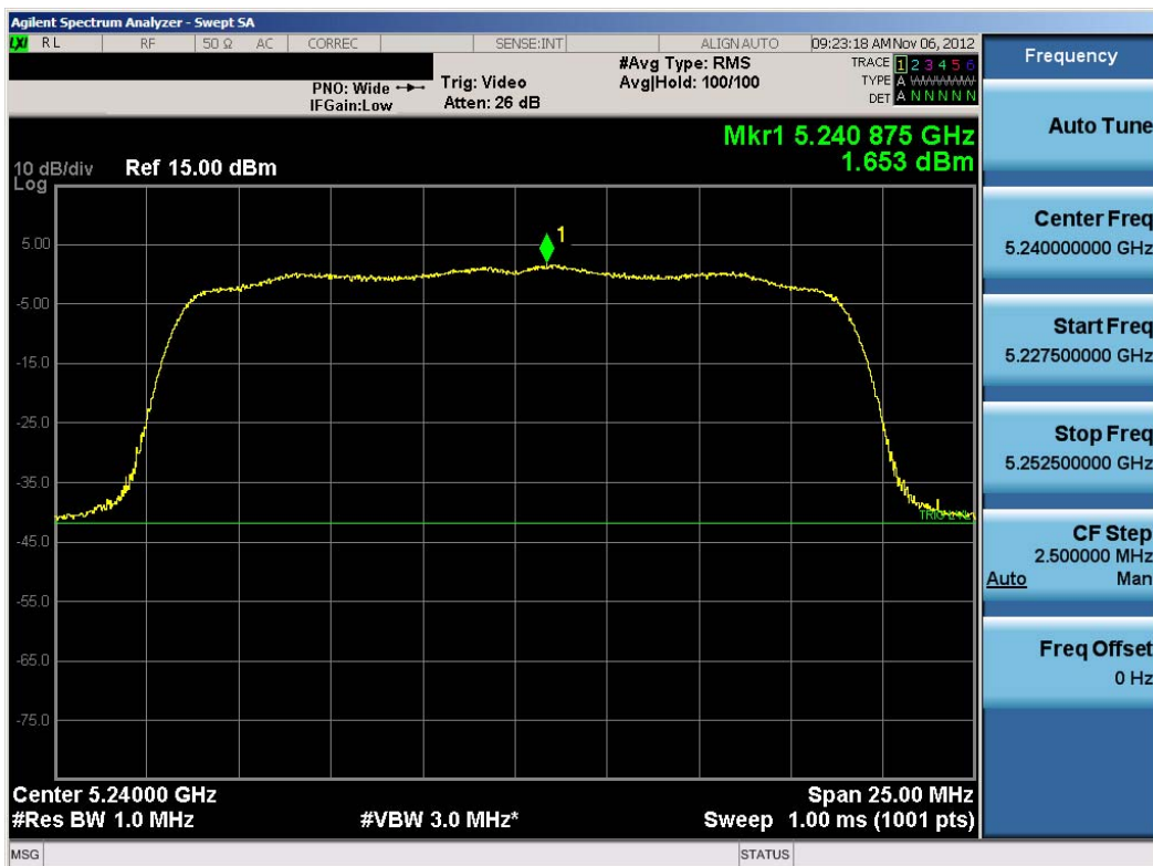
Plot 6-31. Peak Power Spectral Density Plot (20MHz BW 802.11n (UNII Band 1) – Ch. 48)
