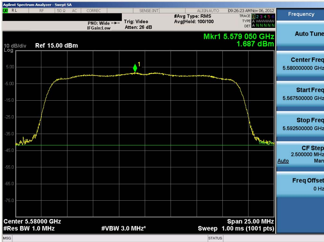
Plot 6-46. Peak Power Spectral Density Plot (20MHz BW 802.11n (UNII Band 3) – Ch. 116)
