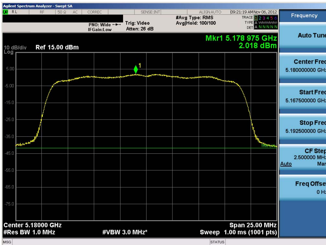
Plot 6-29. Peak Power Spectral Density Plot (20MHz BW 802.11n (UNII Band 1) – Ch. 36)
