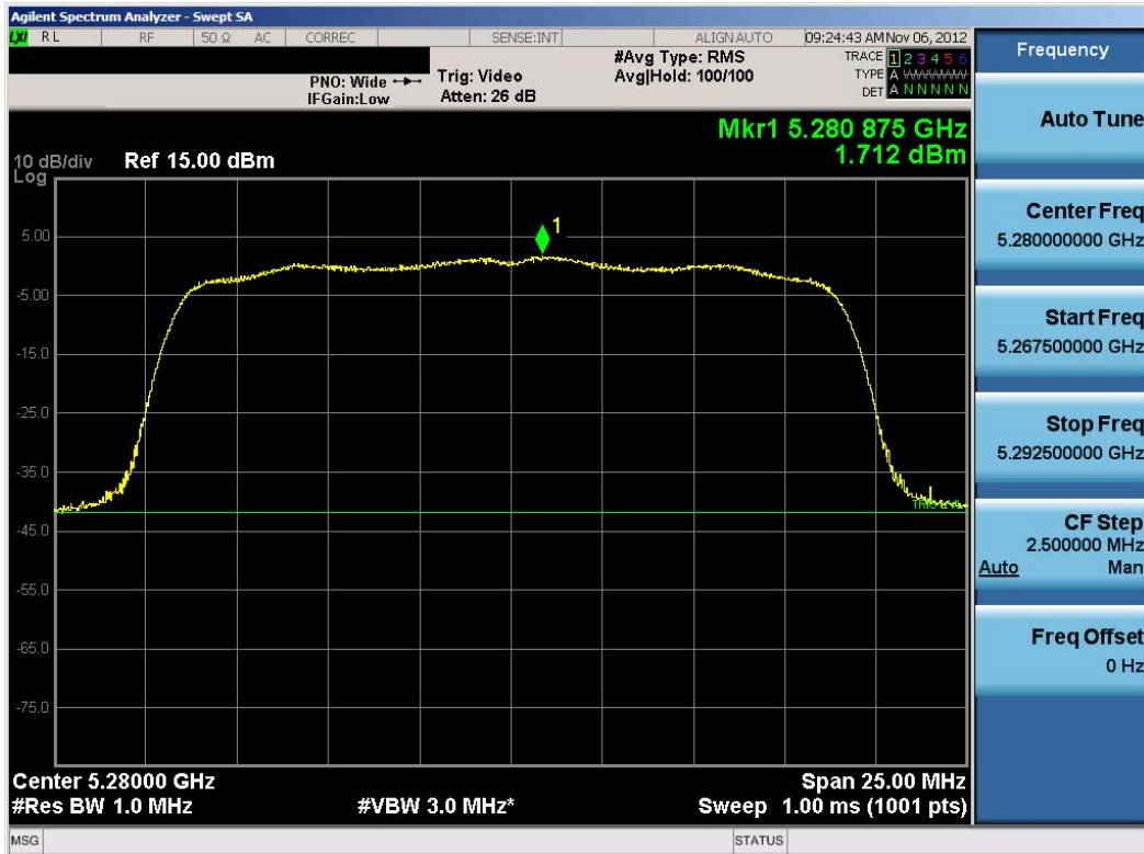
Plot 6-38. Peak Power Spectral Density Plot (20MHz BW 802.11n (UNII Band 2) – Ch. 56)
