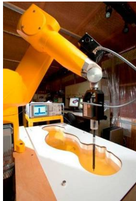
Figure 3-1 SAR Measurement System
