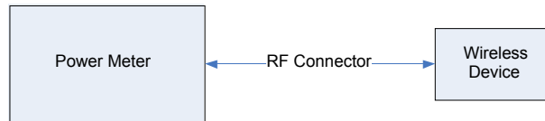
Figure 8-2 Power Measurement Setup
