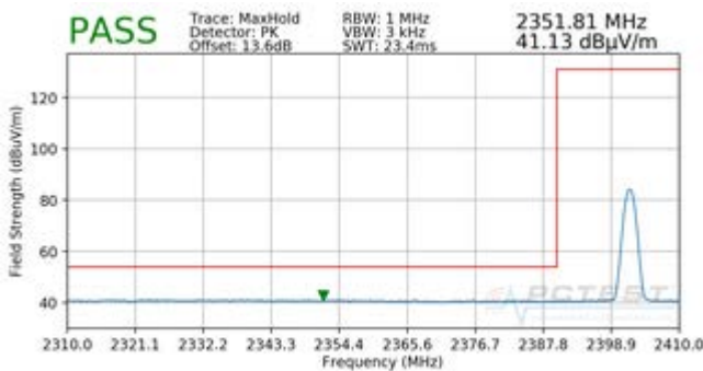
Plot 7-22. Radiated Restricted Lower Band Edge Measurement (Average)
