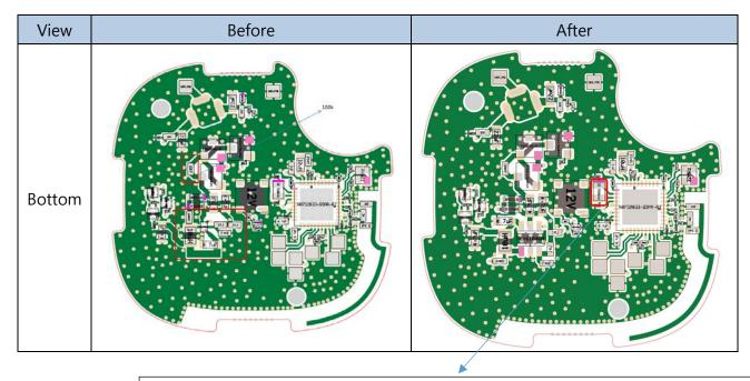
32.768kHz X-tal for BLE IC vendor is added(Seiko Instrument, 2801A0200065)
