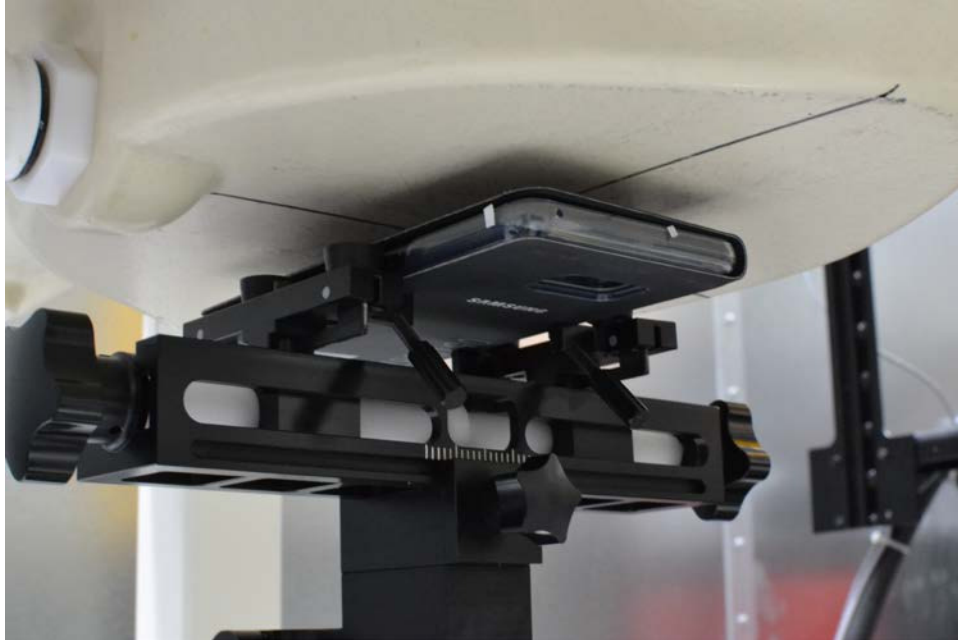
SAR Test Setup Photo 11: Front Side at 1.0 cm, Cover Closed
