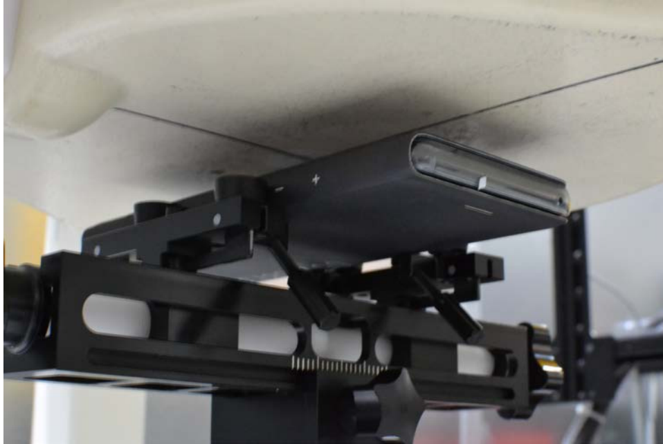
SAR Test Setup Photo 7: Back Side at 1.5 cm, Cover Closed
