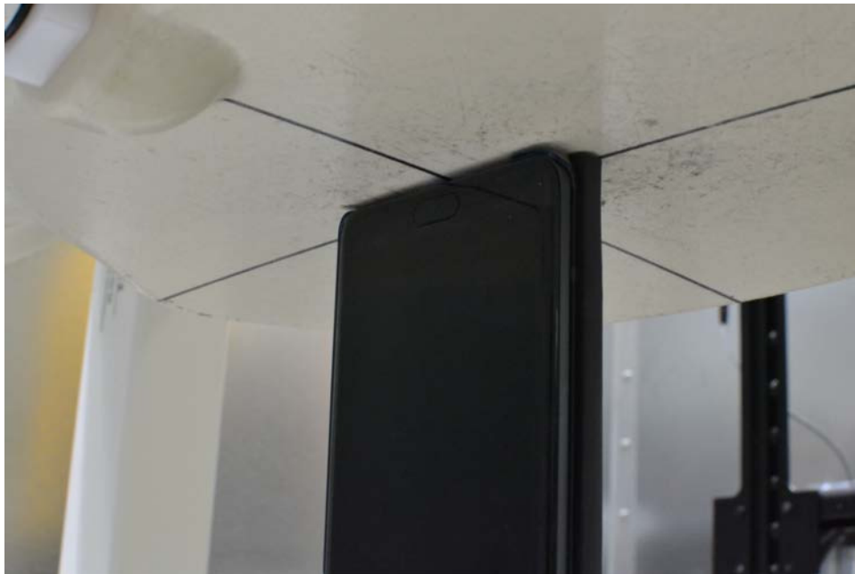
SAR Test Setup Photo 16: Bottom Edge at 0.0 cm, Cover Open
