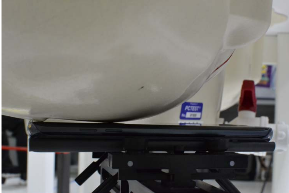
SAR Test Setup Photo 1: Right Cheek, Cover Open
