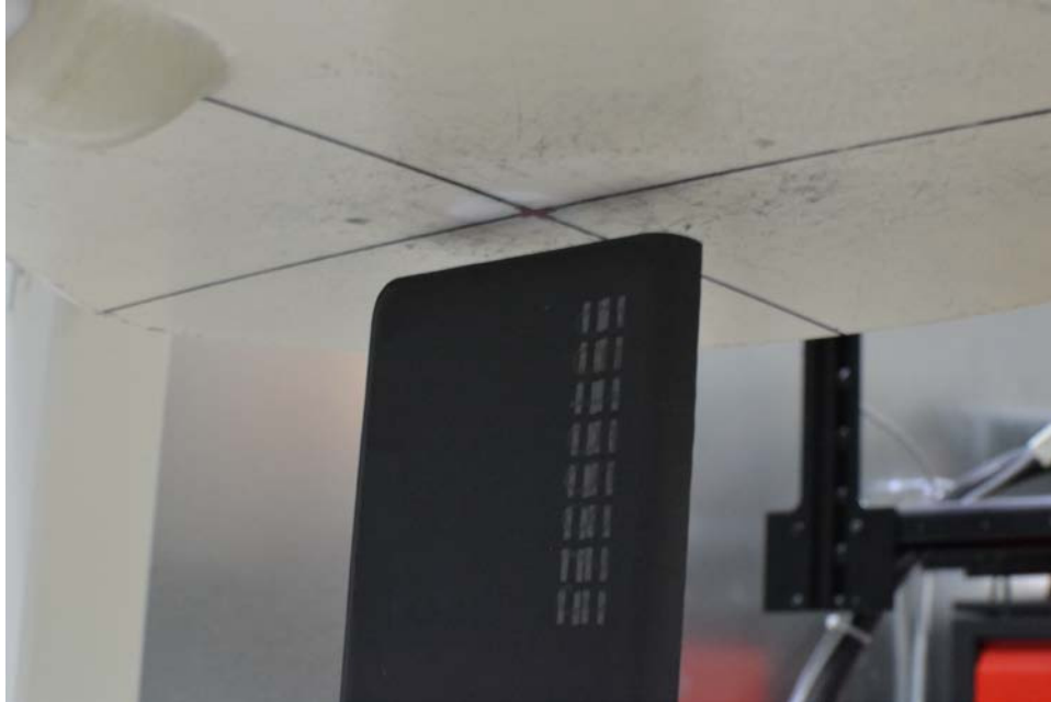
SAR Test Setup Photo 13: Bottom Edge at 1.0 cm, Cover Closed
