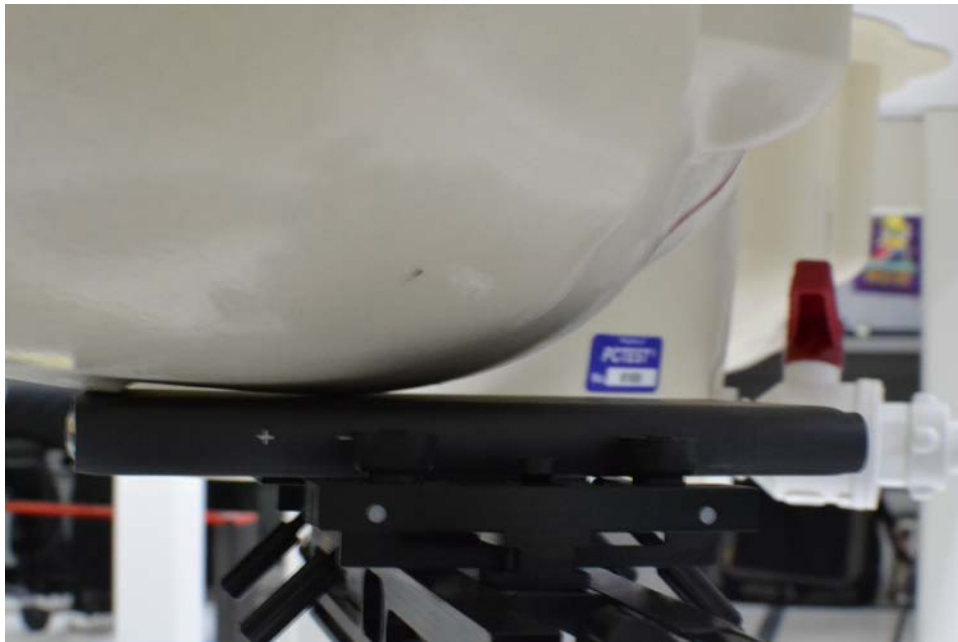
SAR Test Setup Photo 2: Right Cheek, Cover Closed
