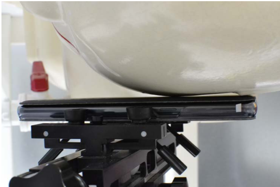
SAR Test Setup Photo 6: Left Cheek, Cover Closed
