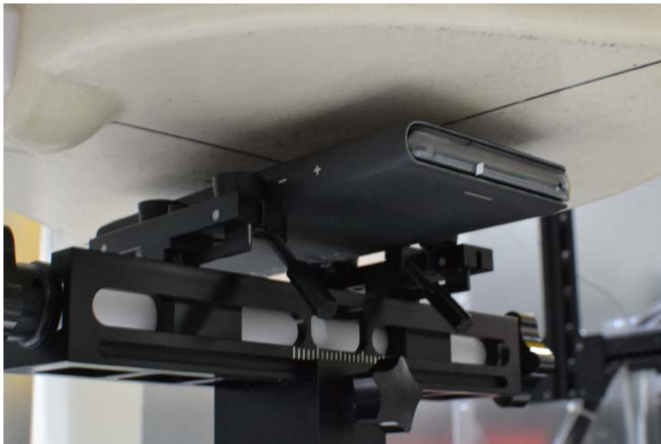
SAR Test Setup Photo 8: Back Side at 1.0 cm, Cover Closed
