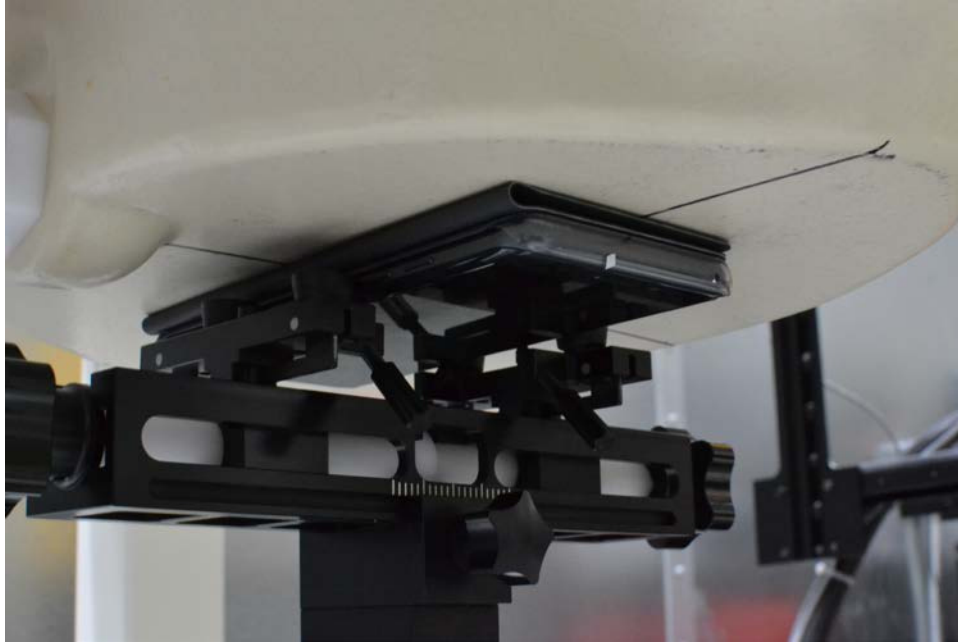
SAR Test Setup Photo 9: Back Side at 0.0 cm, Cover Open
