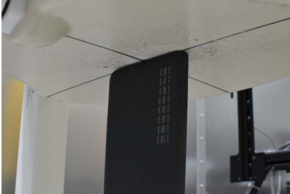
SAR Test Setup Photo 17: Bottom Edge at 0.0 cm, Cover Closed
