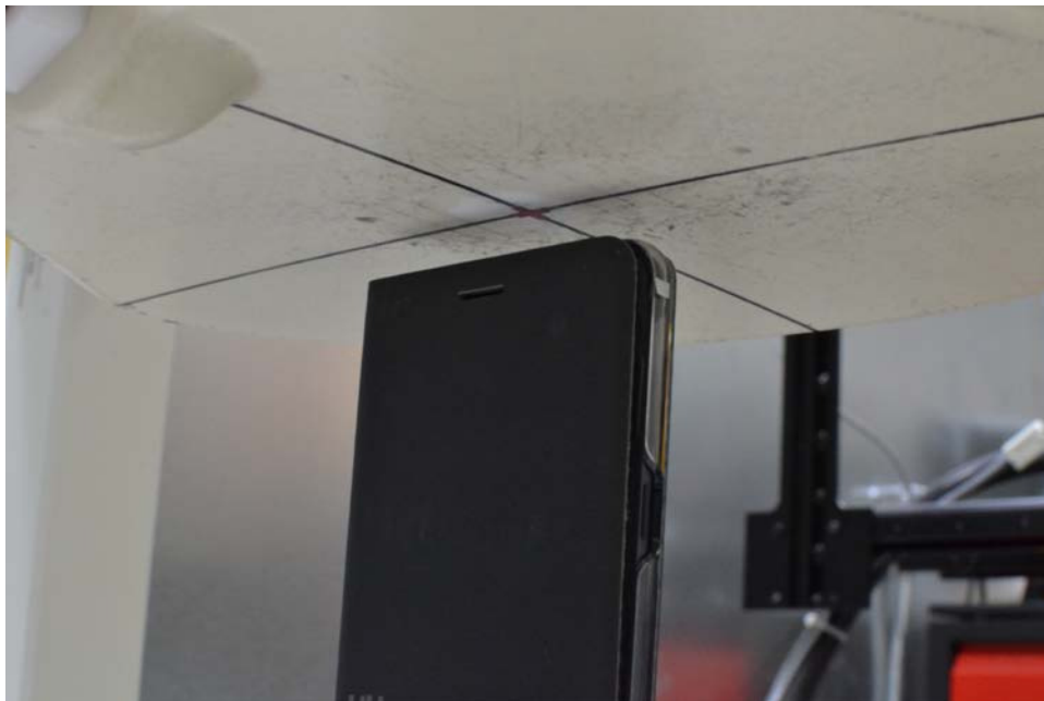
SAR Test Setup Photo 12: Top Edge at 1.0 cm, Cover Closed
