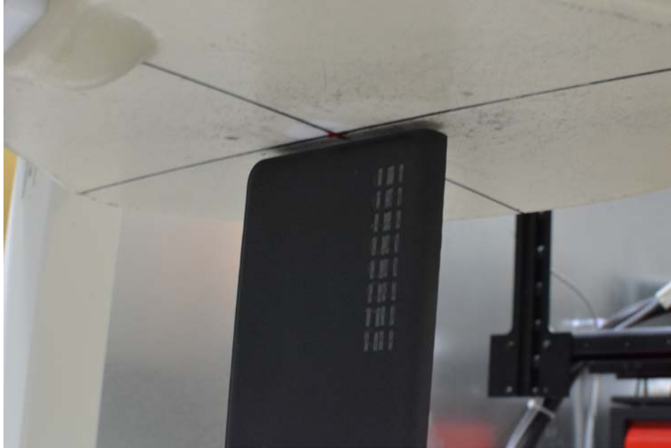
SAR Test Setup Photo 15: Bottom Edge at 0.3 cm, Cover Closed
