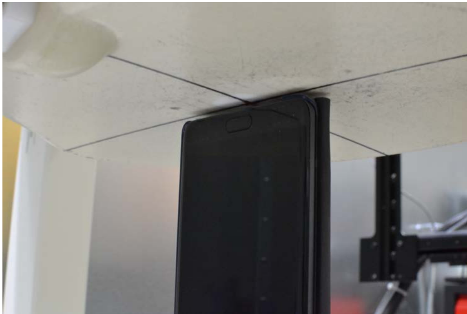
SAR Test Setup Photo 14: Bottom Edge at 0.3 cm, Cover Open
