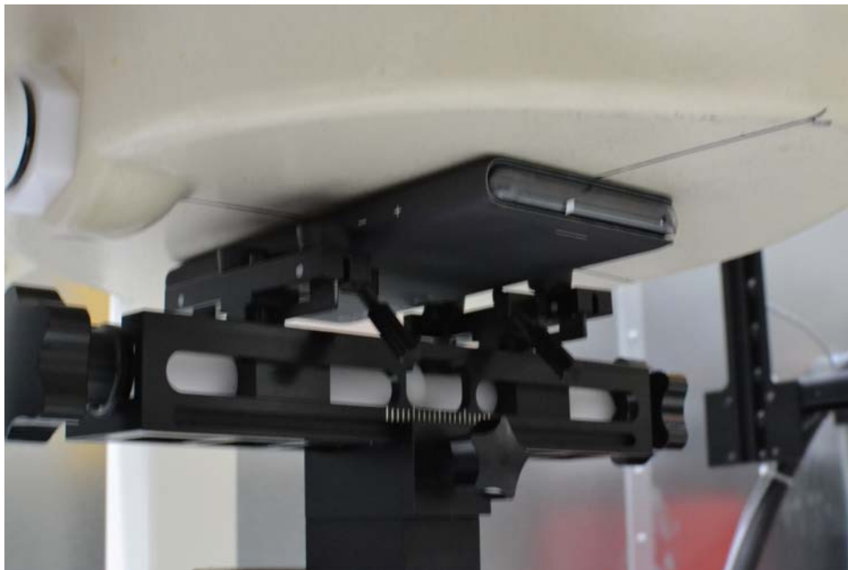
SAR Test Setup Photo 10: Back Side at 0.0 cm, Cover Closed
