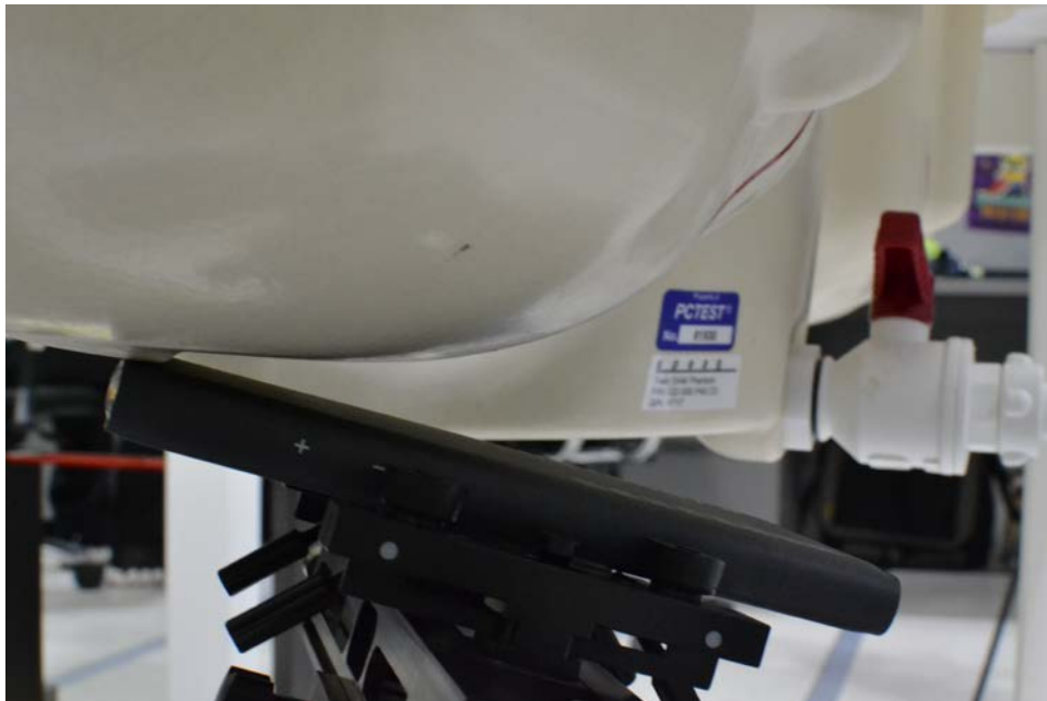
SAR Test Setup Photo 4: Right Tilt, Cover Closed
