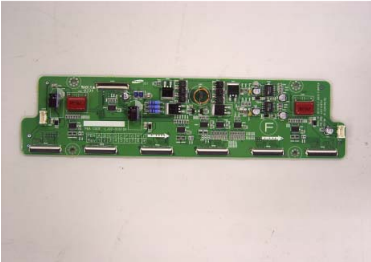
F buffer board top view
