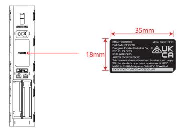
The label is attached to the body of the device under the battery cover with a permanent adhesive.
