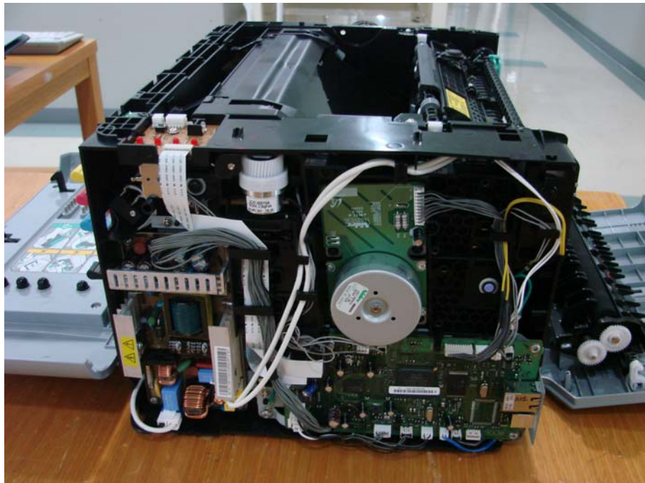
Internal View 4 (with Samsung Electro-Mechanics SMPS board)
